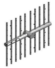
Figure E2. Typical Air Sampling Tree
