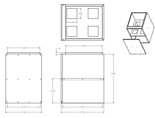
Figure C1. Passive Pressure Drop Device
