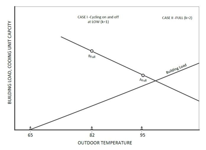
Figure 2. Schematic of a Single-speed System Operation in the Cooling Mode (See Tables 8 and 9 for Temperature References)
