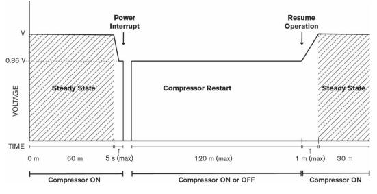
Figure 1. Voltage Tolerance Test Power Interrupt Procedure.
