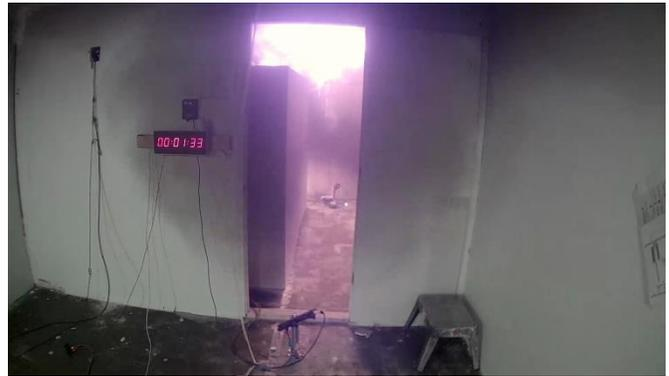
At 85 seconds, the volume around the unit cooler was fully involved in flame and the peak pressure was recorded. This frame shows the peak pressure pushing a plume of smoke out of the walk-in cooler and toward the camera. The total duration of flaming was 58 seconds.
