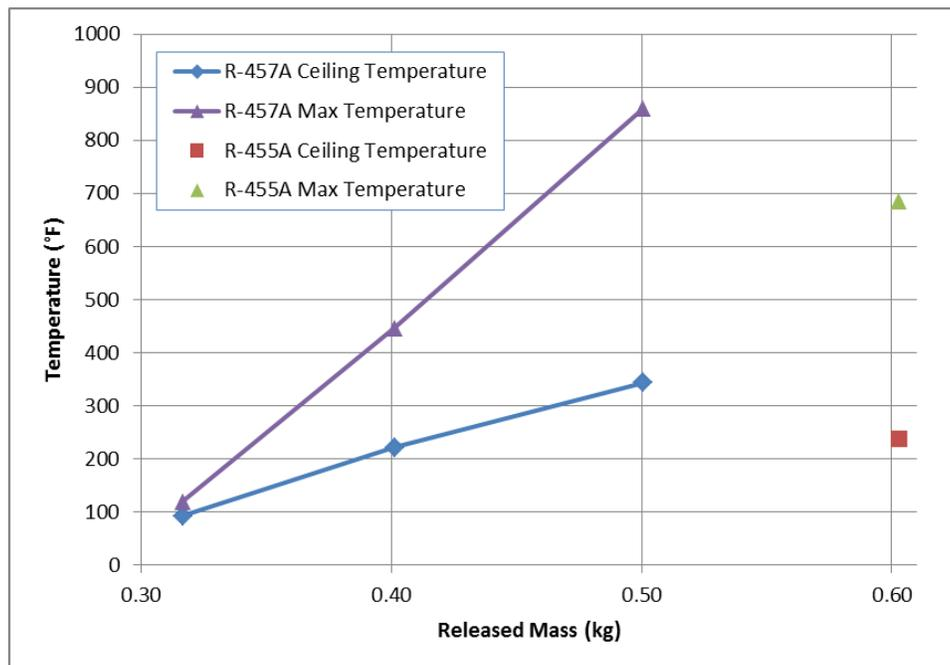
**Figure 107 – Maximum Temperatures and Ceiling Temperatures**
