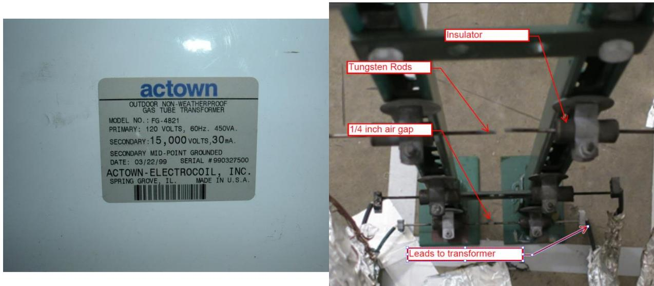
Figure 14 – Gas tube transformer and arc gap
