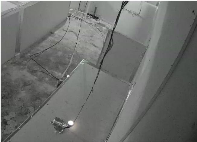
The candle at location C extinguished 30 seconds after the beginning of the discharge. Candle at location D extinguished at 64 seconds (2 seconds after the blower was started). The candle at location A extinguished at 204 seconds. The candle at location B remained lit throughout the test. The candles were observed to flare up at 20 seconds after the beginning of the discharge.
