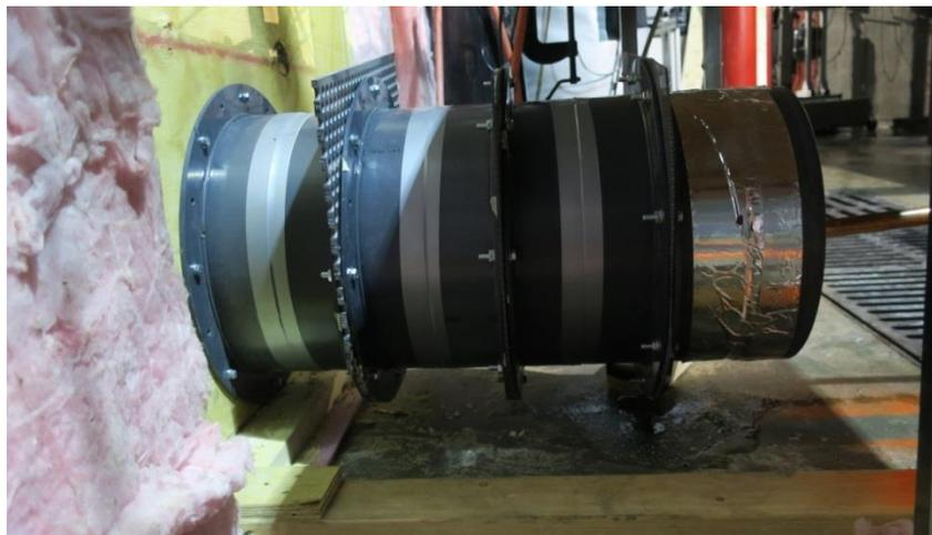
**Figure 19 – Photograph of the 14 in. Duct Assembly**
