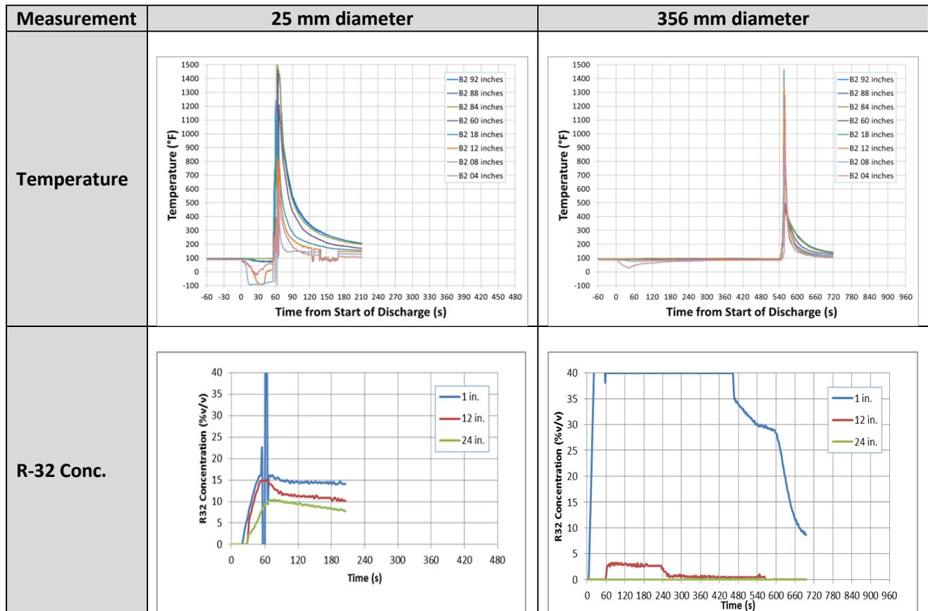
**Figure 40 – Influence of Refrigerant Release Opening Diameter
