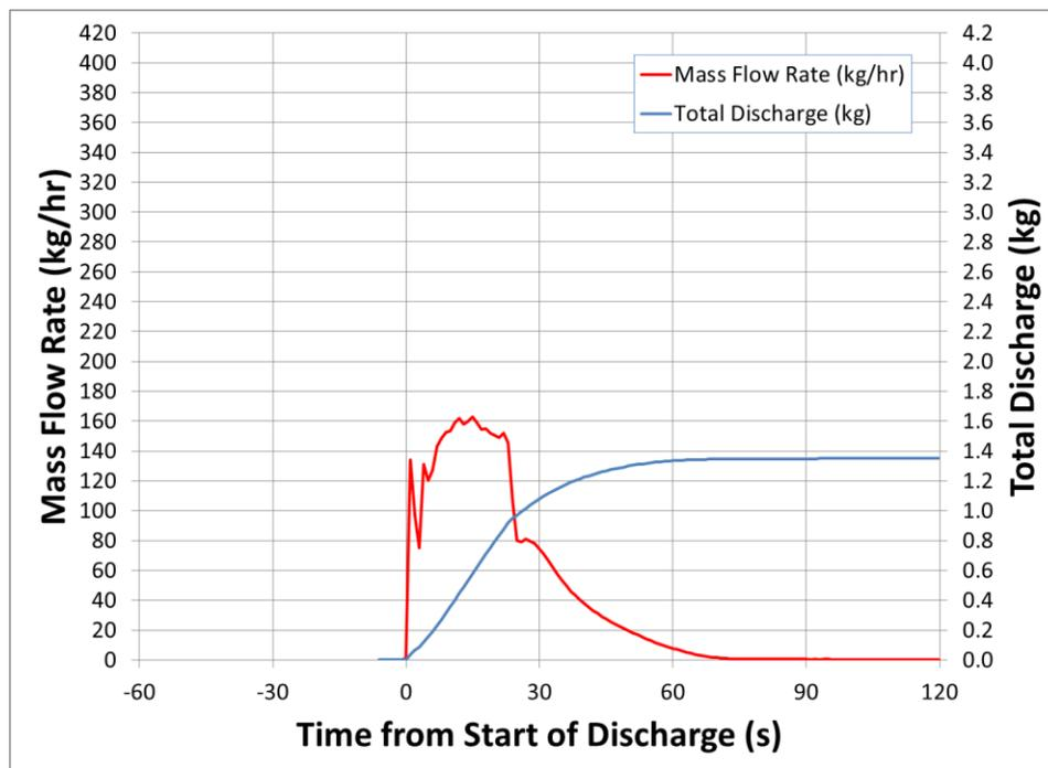
**Figure 145 - Refrigerant Release Rate (RES08 test)**
