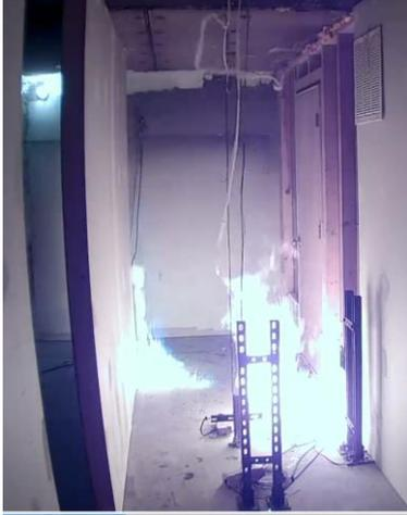
27s after refrigerant release; flame spread observed on the floor in the hallway toward the right wall.
