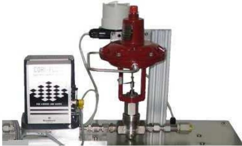
**Figure 164 - Other\Mass Flow Control System**
