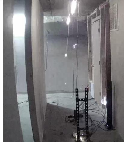
60s after refrigerant release; cheese cloth ignition all the way to the ceiling; all flaming ceased 76s after refrigerant release.
