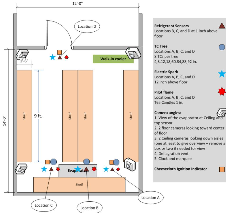
Figure 125 – Larger view of Walk-in cooler detail
