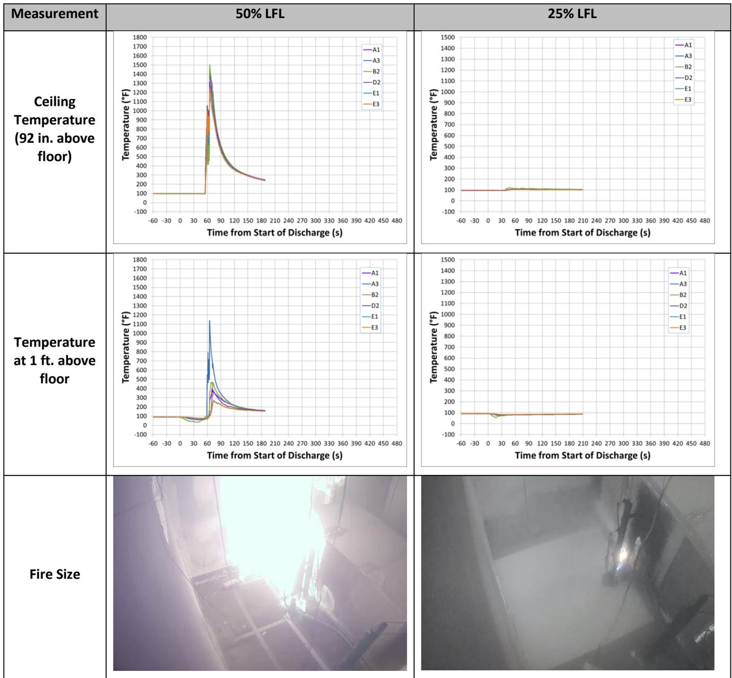
Figure 58 – Comparison of Released Refrigerant Quantity for R-452B Refrigerant
