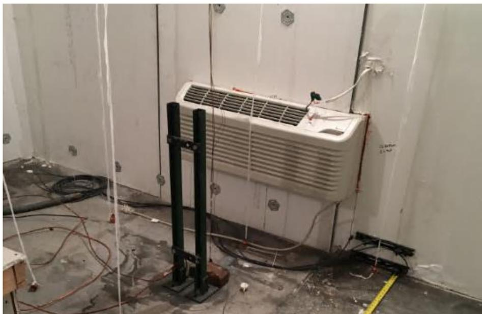
Figure 89 - Camera view of PTAC mounted in the center of the wall
