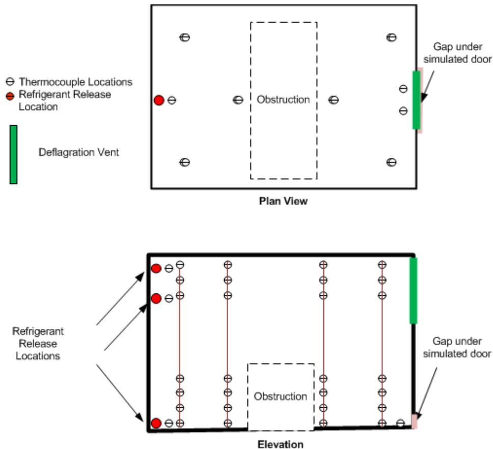
**Figure 13 – Thermocouple Locations Relative to Refrigerant Release**
