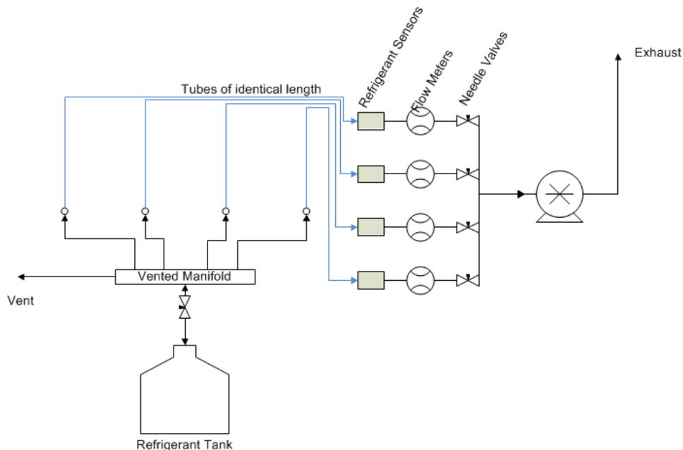
Figure 25 – Setup for calibration of refrigerant sensors
