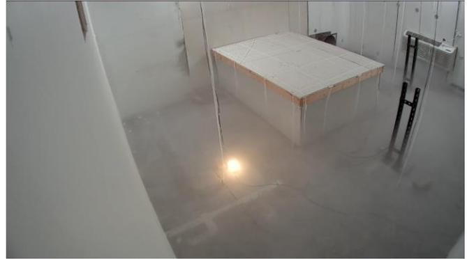
Ceiling camera view at ignition of candles and electric arcs 74 seconds after the start of discharge. Ignition time was delayed by 54 seconds to give time for the technician to leave the test room after closing the manual discharge valves.
