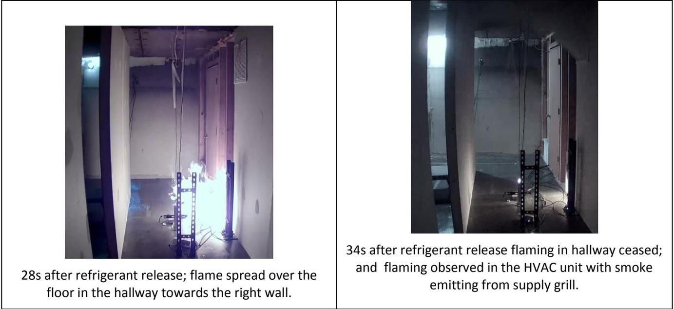
**Figure 139 – Test Results for Residential A/C Test Res02**
