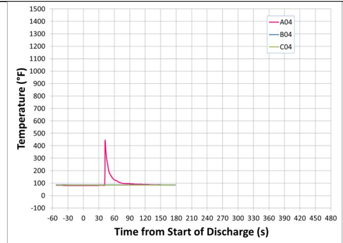
Highest temperature: Temperature 4 in. height above the floor (Location A)
