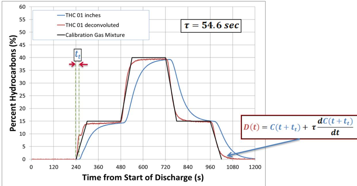
**Figure 27 – Deconvolution test at 0%, 15%, and 40% concentrations**
