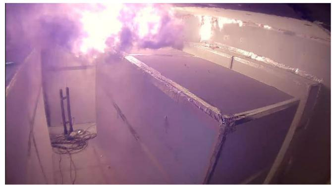
Ceiling level view of flames at ceiling height 105 seconds after that start of the discharge.
