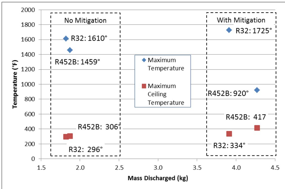
Figure 138 - Peak temperatures near floor and at ceiling
