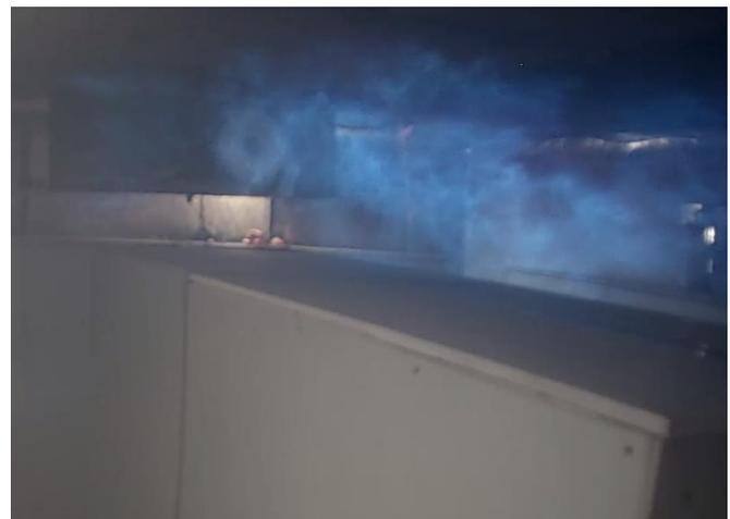
One second after the start of sustained ignition, the flames reached the ceiling of the walk-in. The total duration of sustained flaming was 9 seconds.
