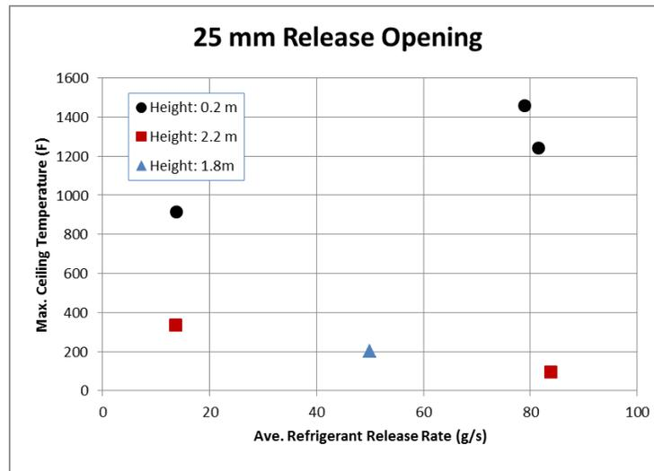
Figure 35 – Maximum Temperature Refrigerant Released from 25 mm diameter opening
