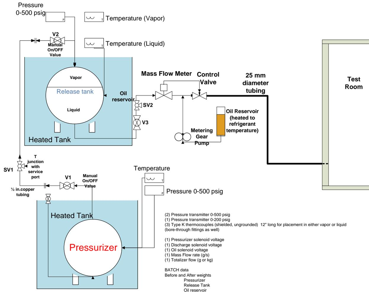
Figure 17 - Refrigerant release methodology with lubricating oil
