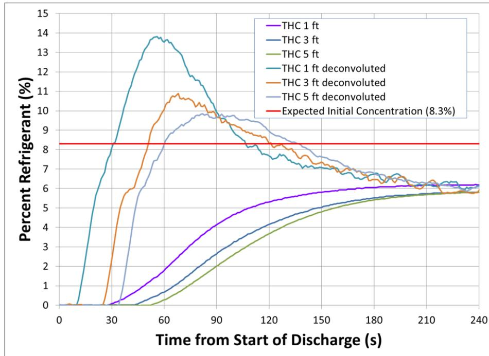
Figure 30 – Deconvoluted concentrations for the room leakage test
