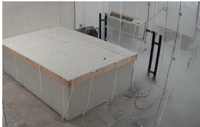
Ceiling camera view 10 seconds after the beginning of the discharge. While not apparent in a still frame, the video shows that discharge location near the corner of the room is directing the mist away from that corner and drawing in fresh air from above the bed.
