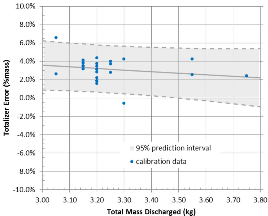
**Figure 22 – Totalizer Error versus Total Mass Discharged**
