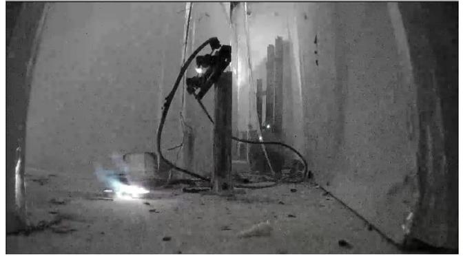
Floor camera view showing ignition at location C, 88 seconds after the start of the discharge.
