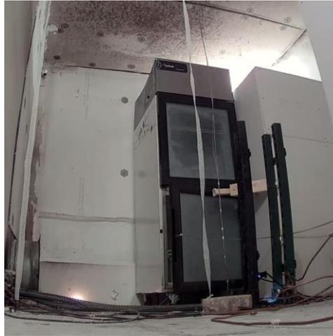
Flaring near pilot flame 5 seconds after the reach-in cooler door was opened.
