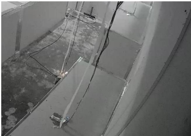
Candle flickering at 34 seconds after the beginning of the discharge. The blower motor had been started 2 seconds prior.
