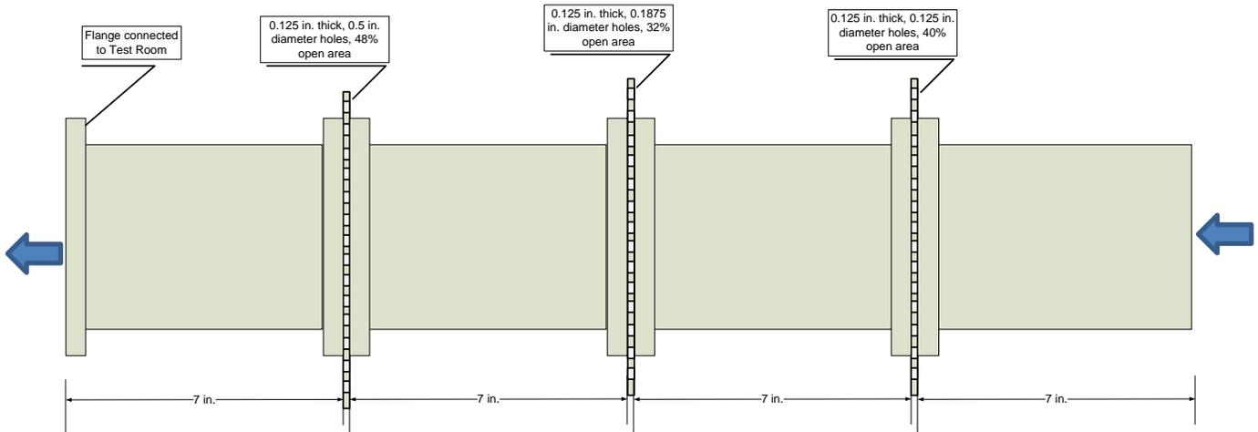
**Figure 18 – 14 in. Release Duct Assembly**
