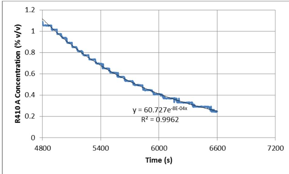
Figure 32 - Refrigerant Concentration Decay with Deflagration Vent Open
