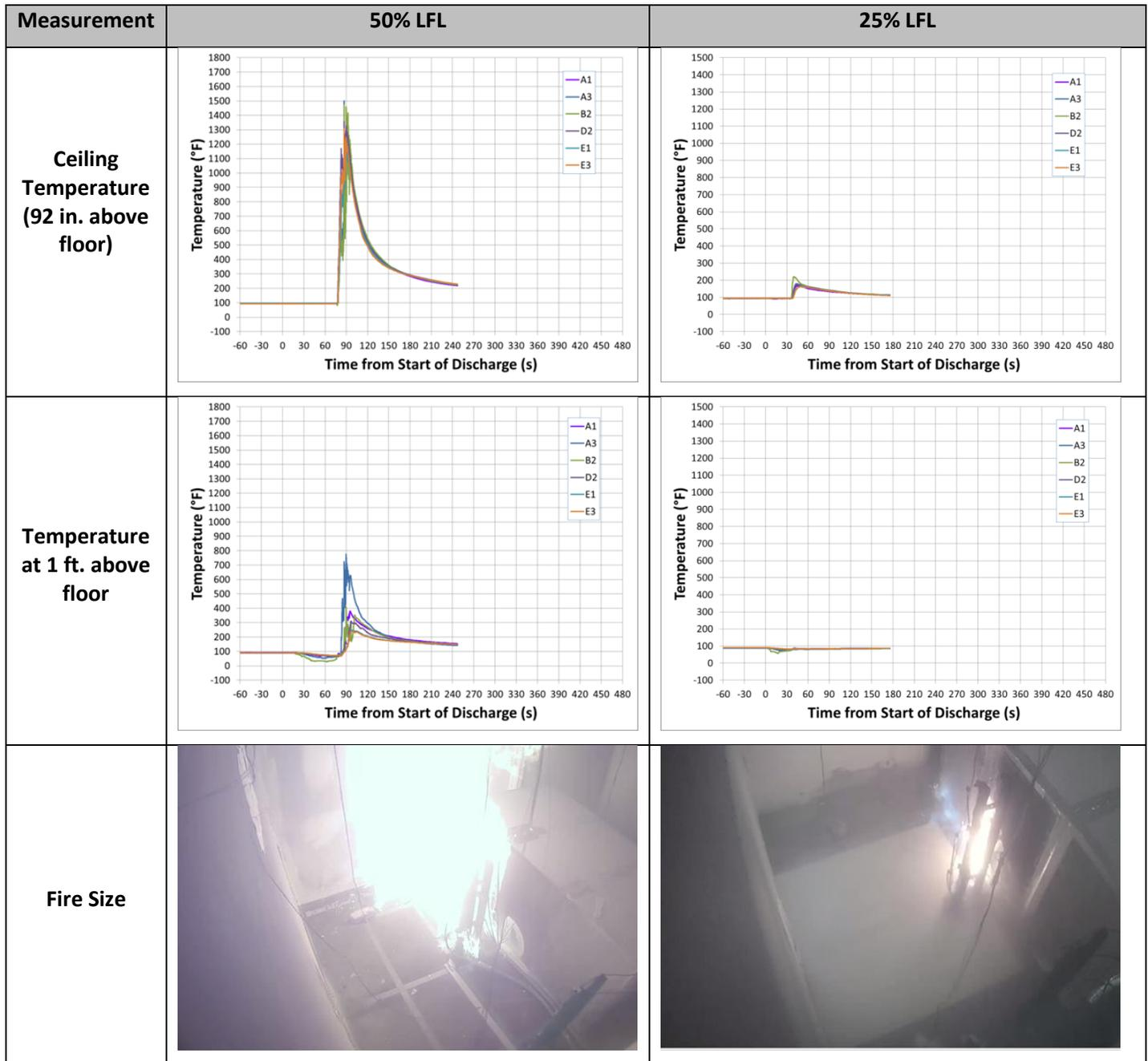
Figure 59 - Comparison of Released Refrigerant Quantity for R-32 Refrigerant
