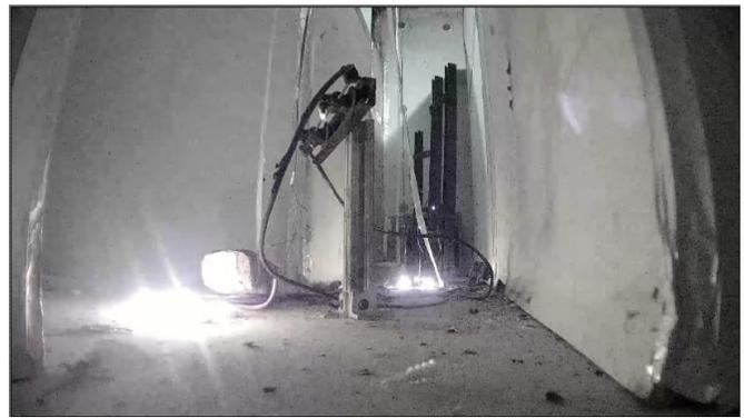
Floor camera view showing flaring at the candles and electric arc at location C and candles at location B.
