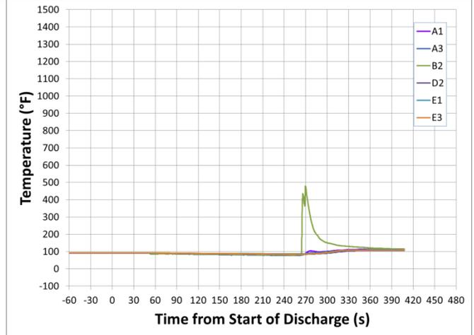
Temperatures at 12 in. height above the floor
