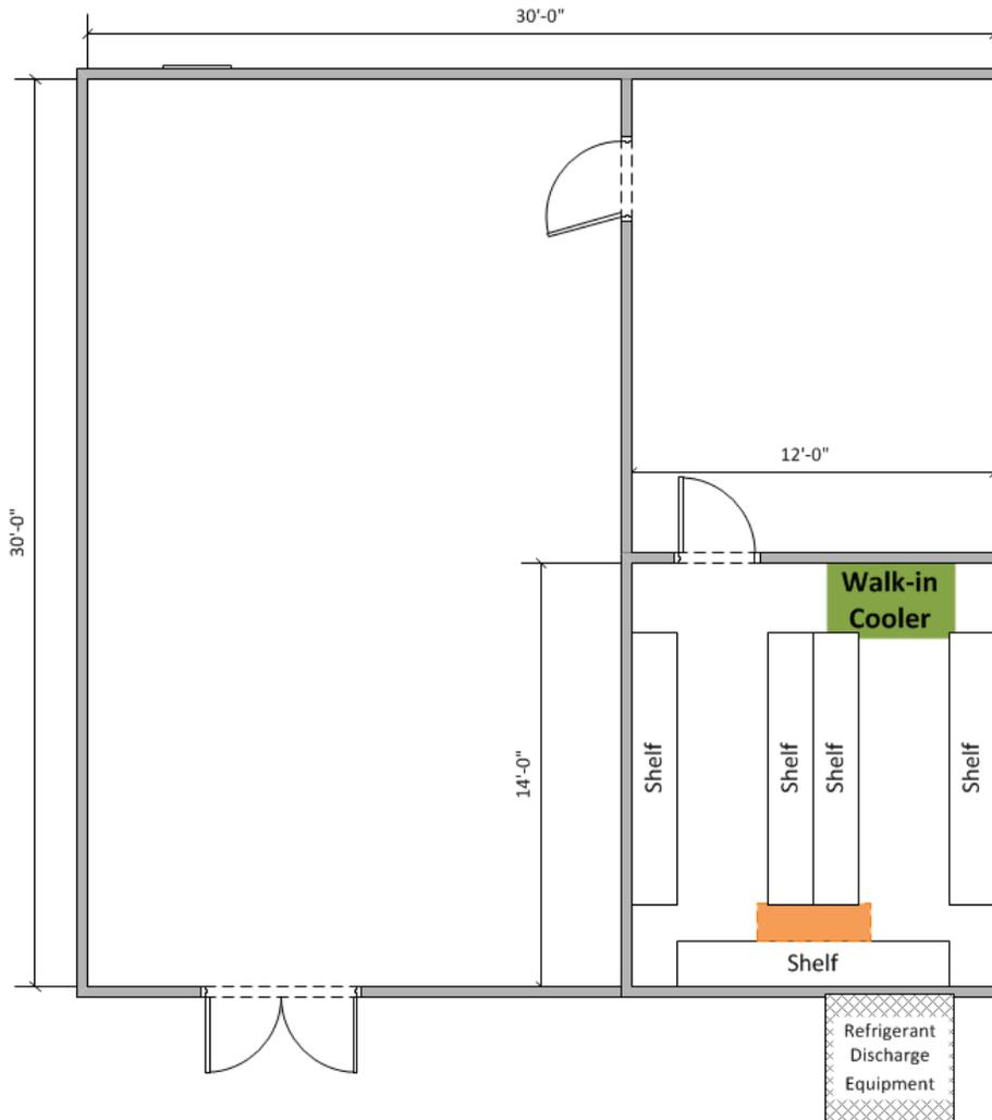
Figure 124 – Walk-in cooler Layout within the 30'x30' test room
