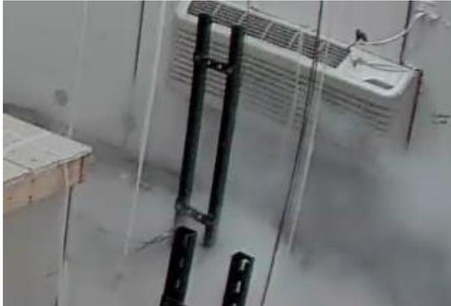
Ceiling camera view at 3 seconds after the start of the discharge. The jet moving to the right was due to the discharge impinging on a vertical support of the grill face.
