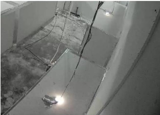
Candles flaring up at 23 seconds after the beginning of the discharge.
