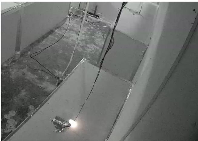
The candles at location B and C flamed out before the beginning of the test. The candle at Location D flared up at 20 seconds after the beginning of the discharge. This candle extinguished 5 seconds later. The candle at location A extinguished at 204 seconds.
