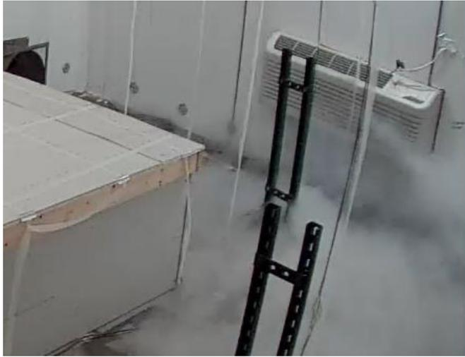
Ceiling camera view at 3 seconds after the start of the discharge. The jet moving to the right was due to the discharge impinging on a vertical support of the grill face.
