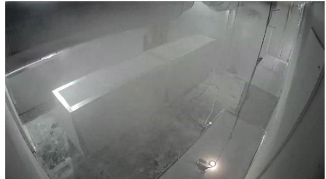
Mist exiting the supply duct at 62 seconds after the beginning of the discharge. The blower motor had been started 2 seconds prior to this frame. The candle at location D extinguished 2 seconds later.
