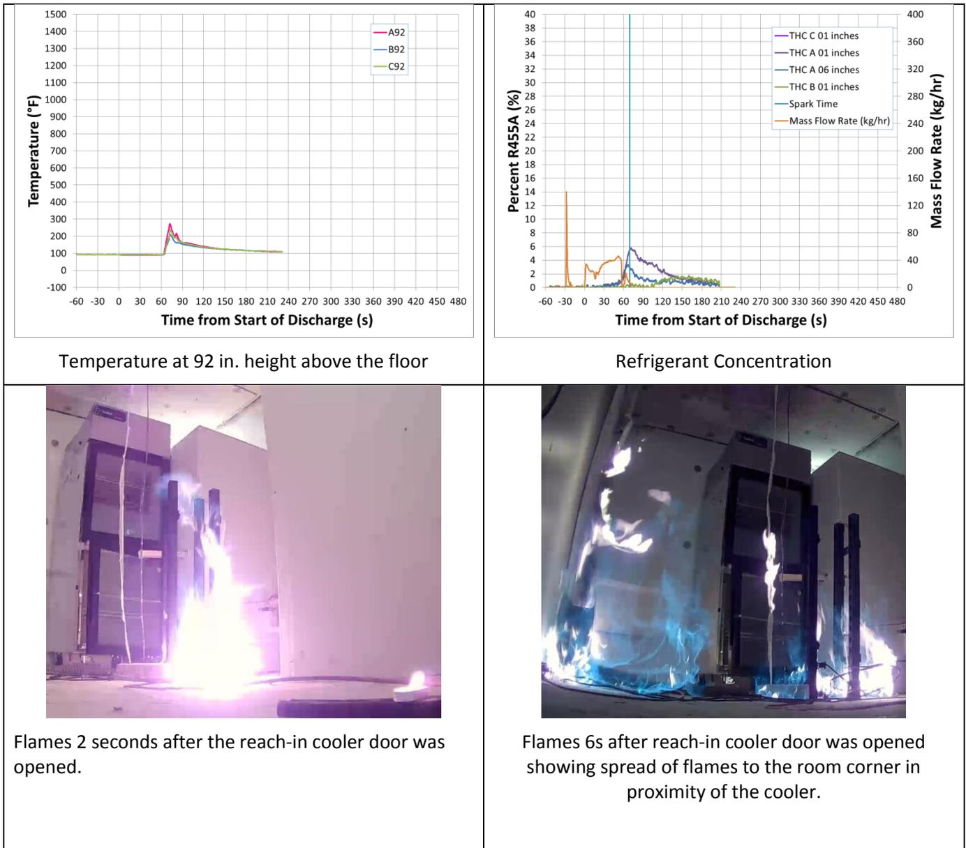
**Figure 108 – Test Results for Reach-in Cooler - Cooler01**
