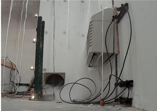
Floor camera view showing additional candles at location A and an additional electric arc at 24 inches. This frame is taken 2 seconds after the start of the discharge.
