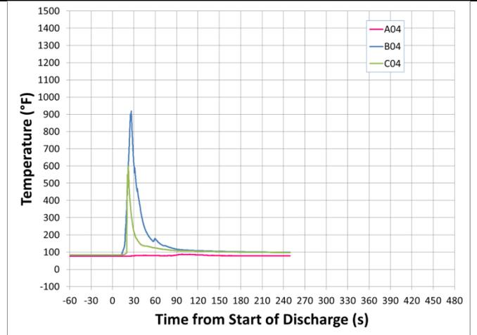
Highest temperature: Temperature 4 in. height above the floor
