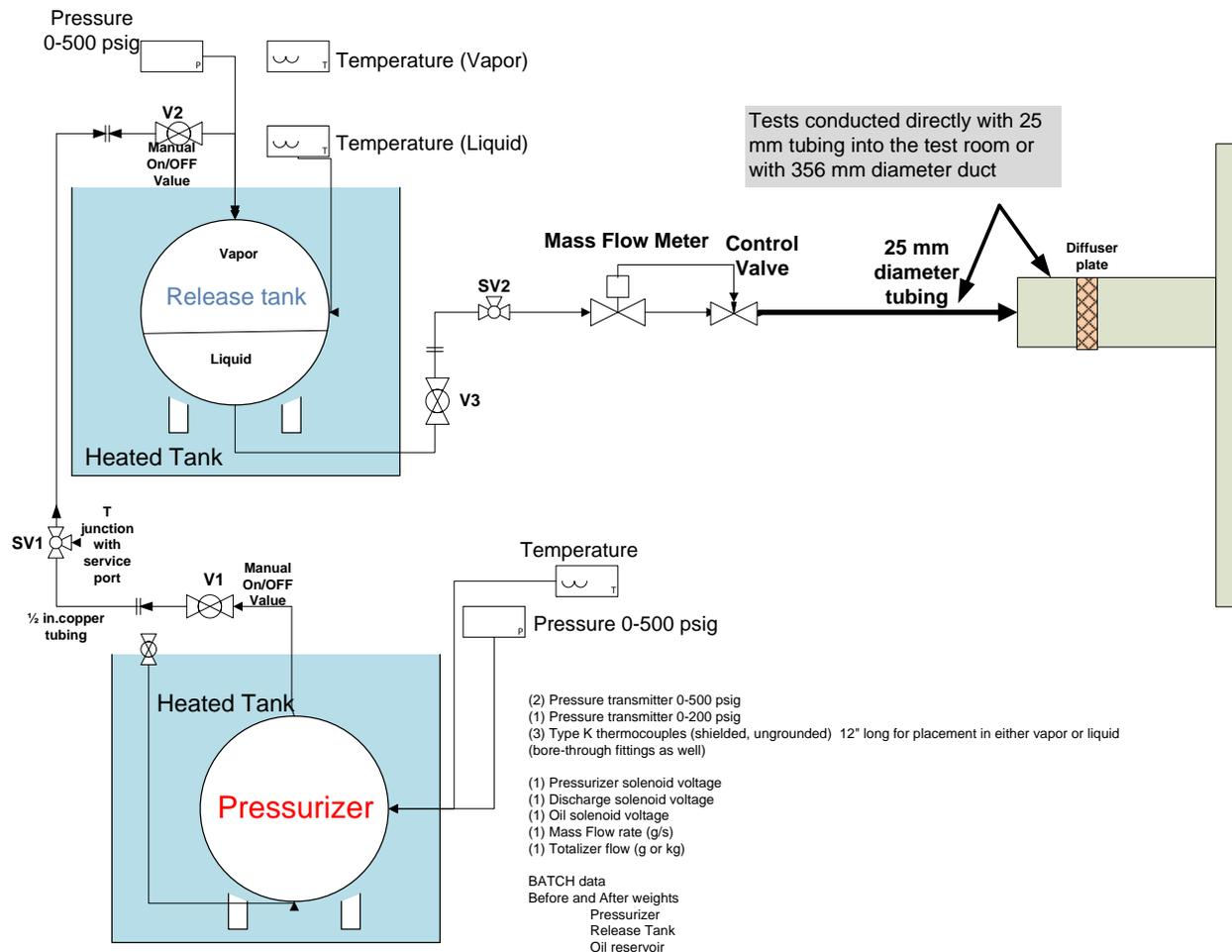
Figure 16 – Refrigerant release methodology without lubricating oil
