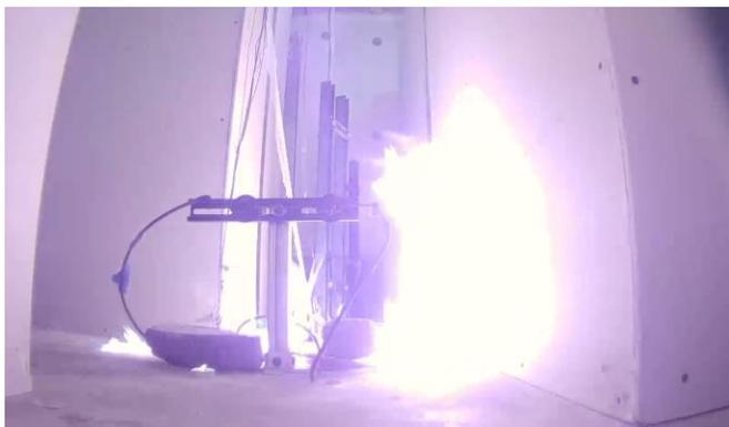
Floor level view at 46 seconds after the start of the discharge. Location C is in the foreground. At 57 seconds the flames reached the ceiling level. Flaming lasted for a total of 87 seconds.
