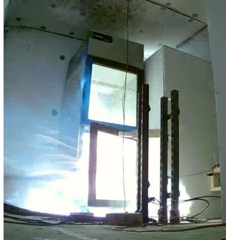
Flames 6s after reach-in cooler door; the flaming spread into the reach-in cooler.
