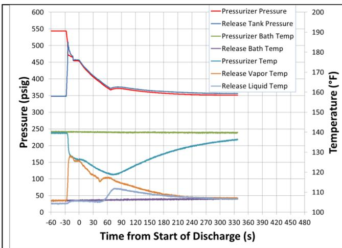
Pressure and Temperature of Release and Pressurizer Tanks
