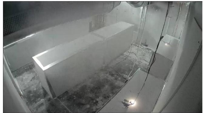
Mist exiting the supply duct at 62 seconds after the beginning of the discharge. The blower motor had been started 2 seconds prior to this frame. Candles at locations C and D extinguished 17 seconds later. The candles at locations A and B remained lighted throughout the test.
