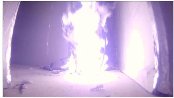
Floor level view at 21 seconds after the start of the discharge. Door was forced open by over pressure 4 seconds later.
