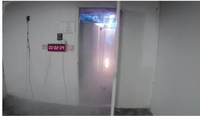
At 61 seconds after the start of discharge, the walk-in door was forced open due to pressure from the ignition.
