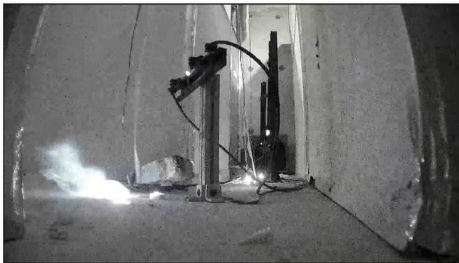
Floor level view at of initial flaming at 13 seconds after the start of the discharge. Localized flaming occurred at the electric arc locations.
