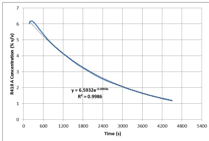
Figure 31 – Refrigerant Concentration Decay with Deflagration Vent Closed
