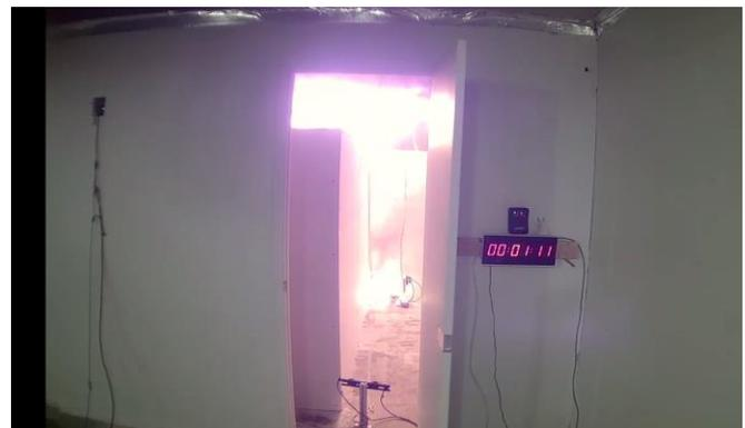
The latch on the door was disabled in order to use the door as a deflagration vent. The door was forced open at 59 seconds after the start of the discharge.
