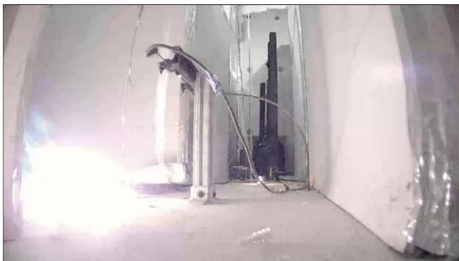
Floor level view at 10 seconds after the start of the discharge. Localized flaming occurred at the electric arc locations.
