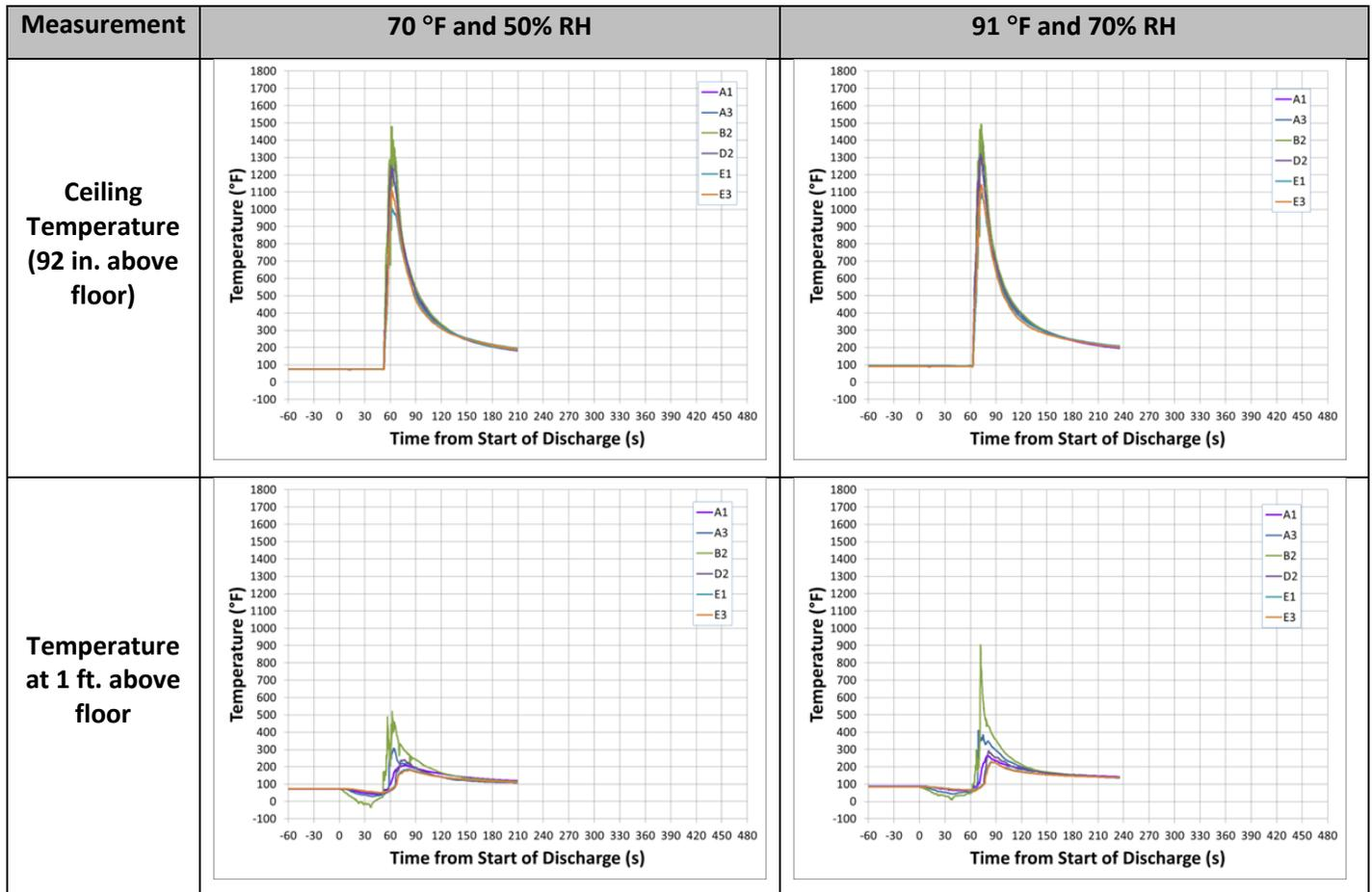
**Figure 54 – Influence of Ambient Temperature and Humidity for R-32 Refrigerant**
