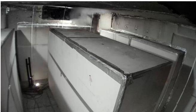
Ceiling camera view of the discharge showing the condensation cloud at the ceiling level.
