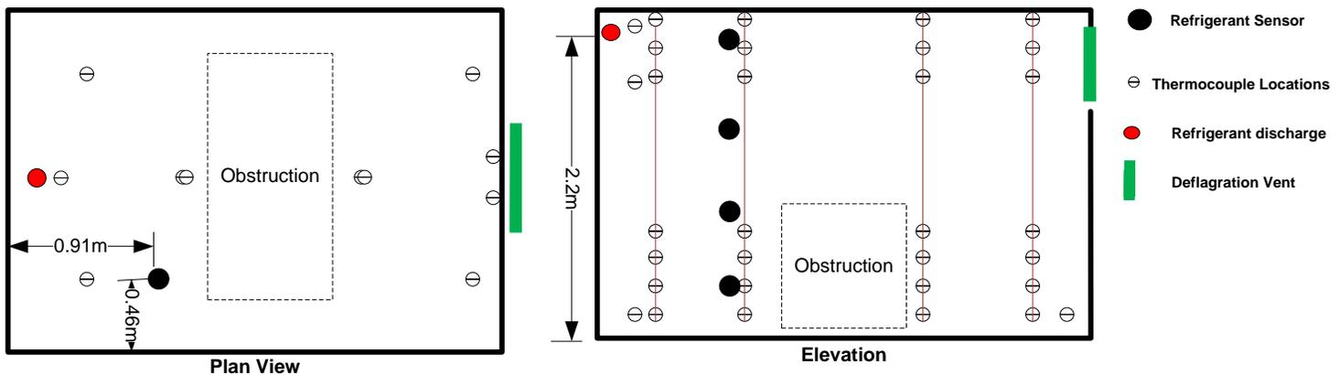
Figure 28 – Test Room Leakage Characterization
