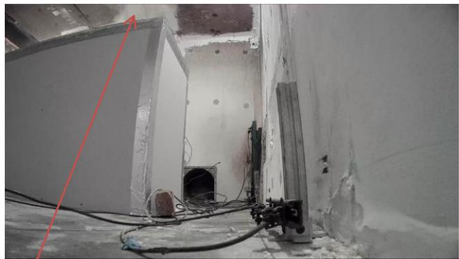
Mist exiting the supply duct at 62 seconds after the beginning of the discharge. The blower motor had been started 2 seconds prior to this frame. Flames about 1 inch in height were observed at the electric arc locations after the blower had been running for 5 seconds.
