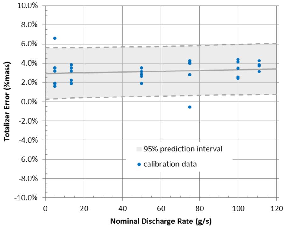
**Figure 23 –Totalizer Error versus Nominal Discharge Rate**
