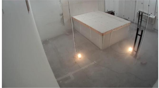
Ceiling camera view at ignition of candles and electric arcs 83 seconds after the start of discharge. Ignition time was delayed by 27 seconds to give time for the technician to leave the test room.
