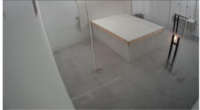
Ceiling camera view at ignition of candles and electric arcs 57 seconds after the start of discharge.
