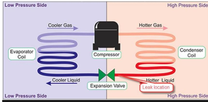
**Figure 10 – Refrigeration Leak Scenario**
