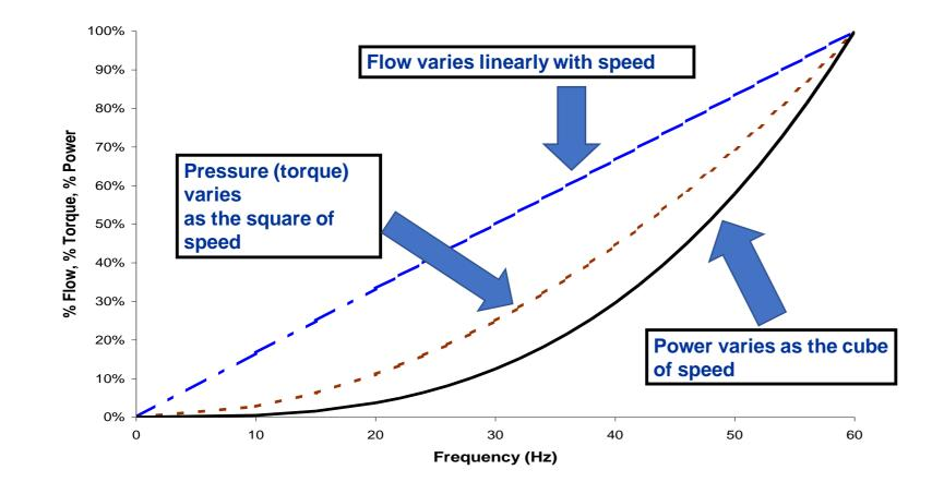
For 100 HP (74.6kW) Application: 80% Speed = 51.2% Power 60% Speed = 21.6% Power 40% Speed = 4.8% Power
