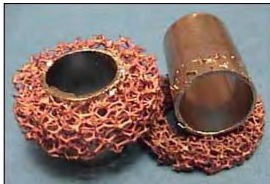
Figure 4.11 Copper foam brazed with Au/In braze alloy (left) and after bond strength test (right) [205]
