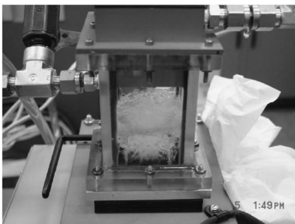
Fig. 3. (a) CMOS chip with the resistors for heating and monitoring temperature. (b) Silicon based CMOS chips bonded to graphite foam blocks. (c) Bond chips inserted into the PGA. (d) Wire bonded PGA package. (e) Evaporative chamber mounted to PGA package.
