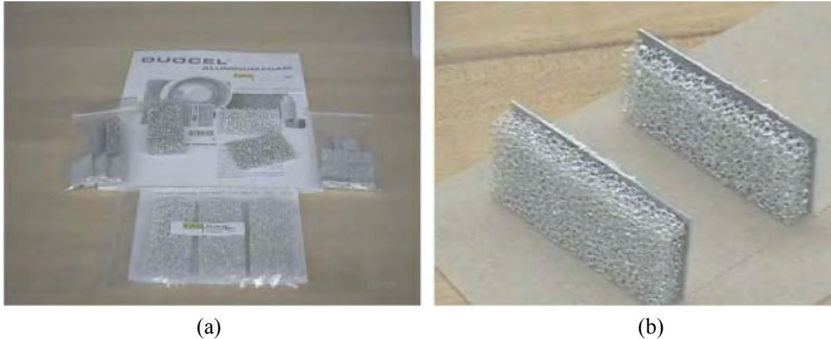
Figure 2.41 (a) Aluminum-foam samples, from Duocel; (b) foams bonded to aluminum substrate [113]
