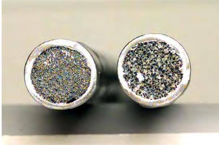
Figure 2.40 Metal-foam filled tubes using co-sintering technique. [107]
