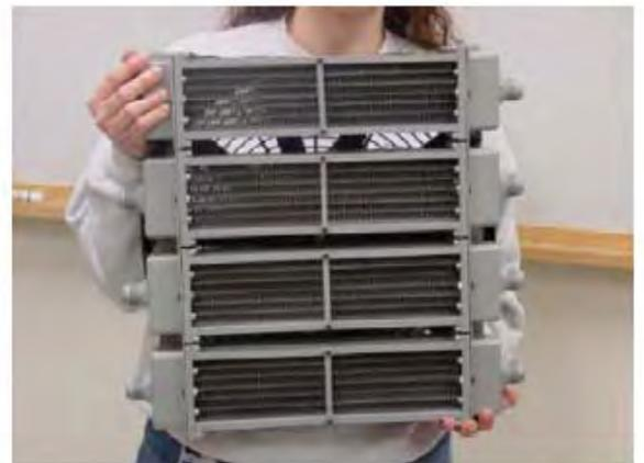
**Figure 3: Automotive radiators which demonstrated 33 to 250% performance improvement.**
